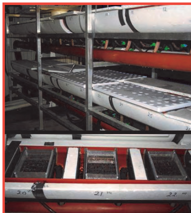
Figure 1. Experimental units for hatching of rainbow trout eggs. The units have individual inlets and outlets and, each unit is insulated to insure stable temperatures.
